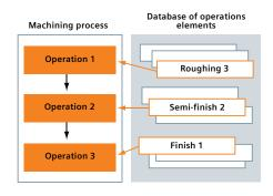
You can easily configure, add or modify the feature-based machining operations and how they are selected using a simple editor (Machining Knowledge Editor).
